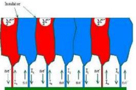
The SentinelCorr™ CRC system combines the capabilities of the SentinelCorr™ CR system with capabilities to measure pH, chloride, and temperature all in a single probe. Like the CR system, the CRC can measure both general and localized corrosion. Corrosion is measured by funneling the electrons passed between anodic and cathodic sites on the corroding surface discrete channels, where the current magnitude and direction (flowing to or away from that electrode) can be determined. This is
